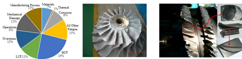
Fig. 5. damages of structure and disc fatigues due to vibration
