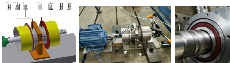
Fig. 23. A rotor test-rig supported by two bearings
