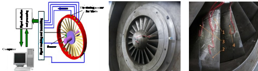
Fig. 19. The measuring system of blade vibration and crack
