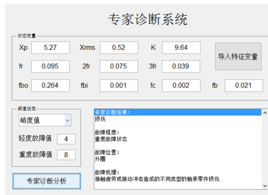
Fig. 28. Interface of an ES based fault diagnosis for bearing faults
