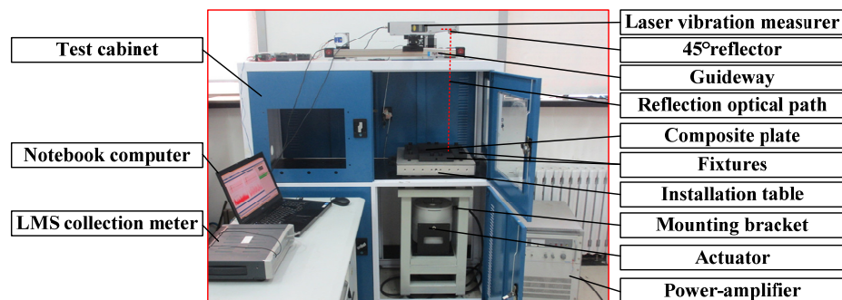
Fig.2. Picture of the modal parameter testing system of fiber-reinforced composite plate
