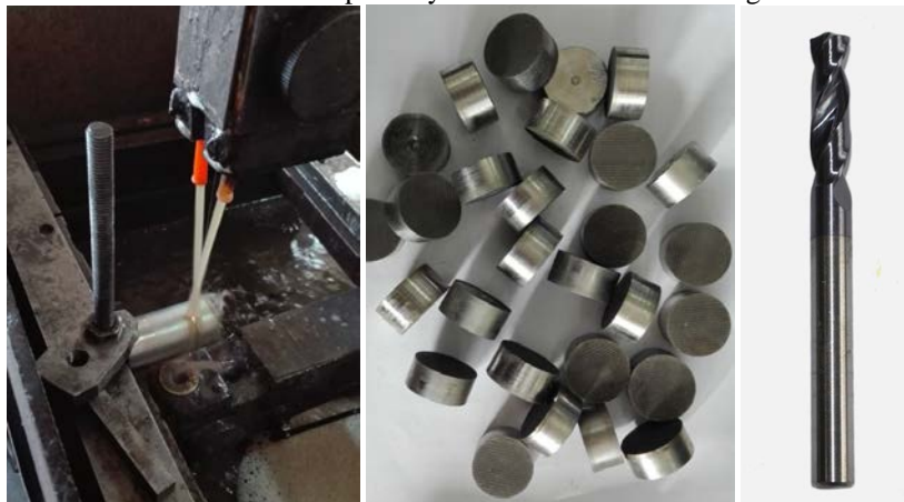
Fig.1. Test specimens of GH4169 Ni-based superalloy and drill
