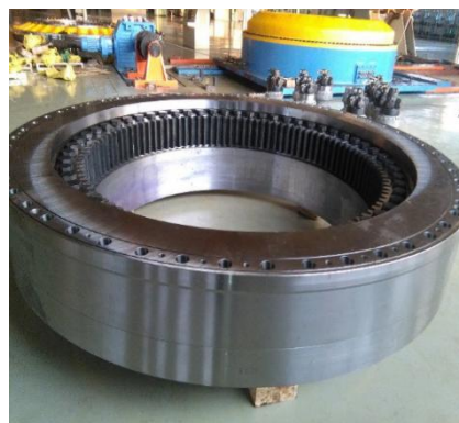
Fig.2. Main bearing in TBM
