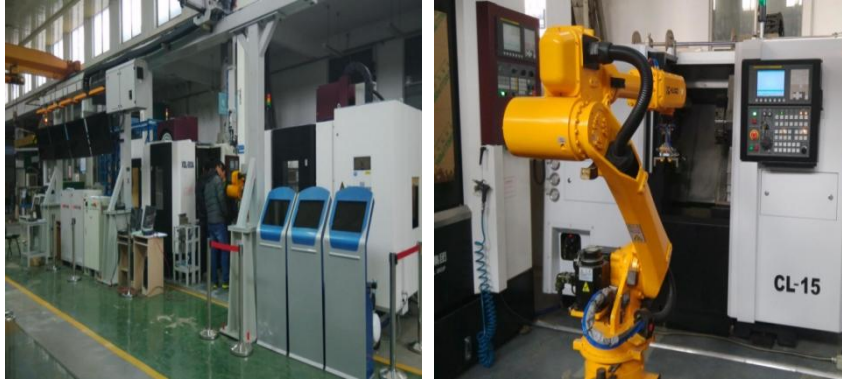
Fig .5. Teaching module based on FMS Flexible Island
