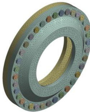
Fig. 3. The meshing of wheel disk assembly
