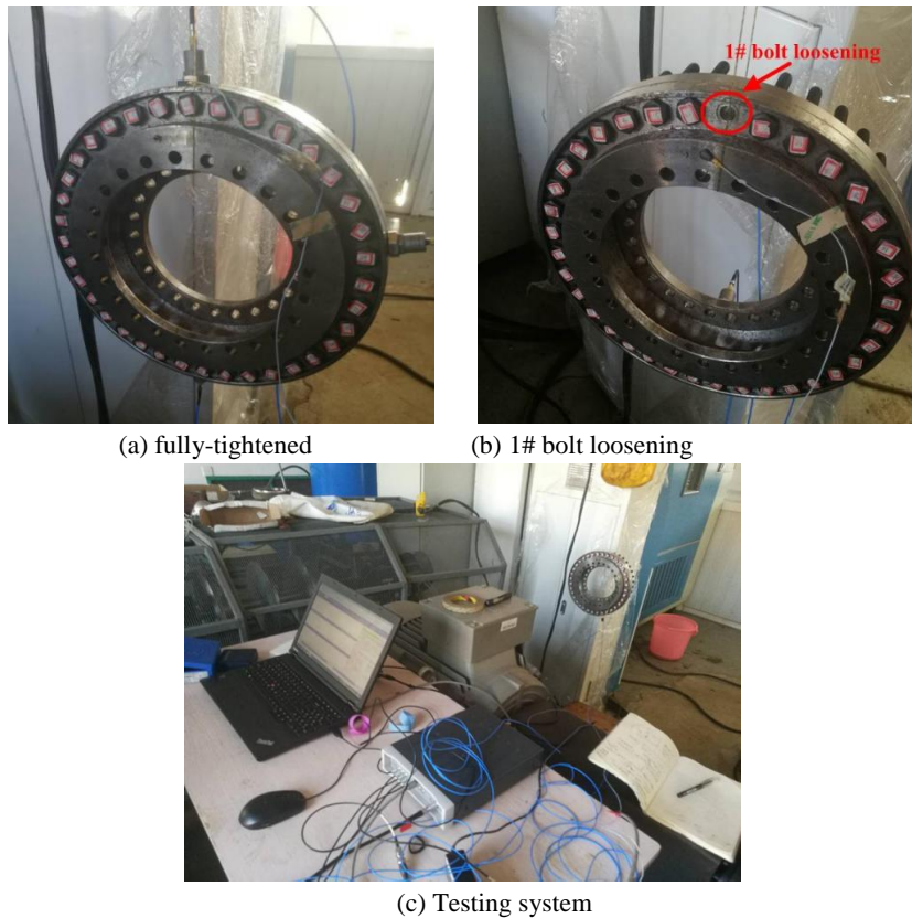
Fig. 8. The photos of test site
