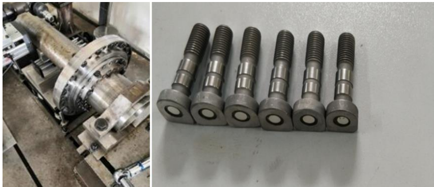
Fig. 8. Experimental specimen and ultrasonic bolt
