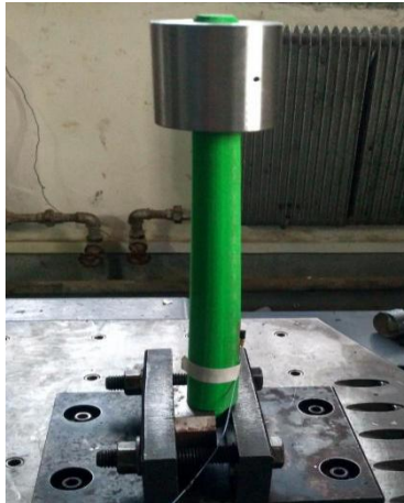
Fig. 13. Frequency Swept Test of Solid Strut-Mass System on Shaker
